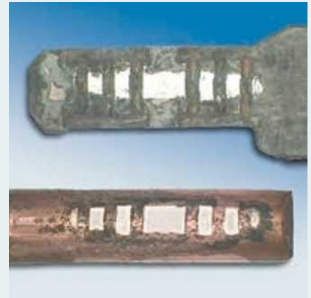
Contact area of a screw terminal block after testing
